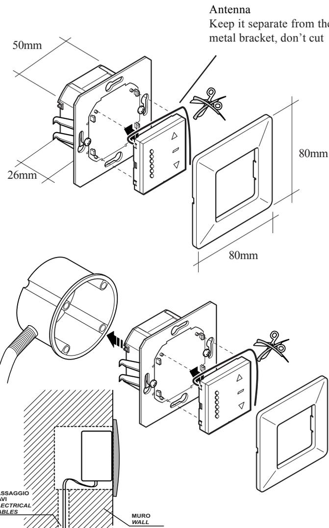
**The appliance must be installed either by means of the fastening screws or the lateral hooks. Strip the wires as little as possible and block them in position near the binding posts using plastic clips. Fasten the wires well so that they cannot slip out of their binding posts.**
